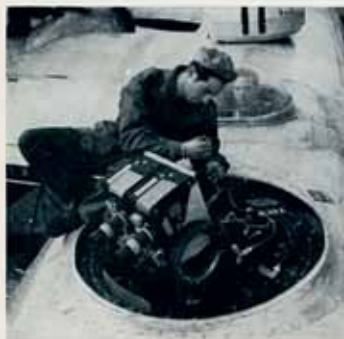
PREFACE TO PRECISION. On a Boeing F-13 plane altered for use as a photographic ship two motion picture cameras are installed in one of the plane's gun turrets. These cameras were controlled from the top fire control blower shown in the background by the same sighting and firing mechanisms normally used with the plane's machine guns. Shows here at Roswell Field, New Mexico, are Corporal Harold Johnson, outside the plane, making adjustments on the camera, while Sergeant Henry R. Zarnoff, near the controls in the top fire control blower. In the background can be seen another turret, started cover in place, housing a similar motion picture camera installation.
